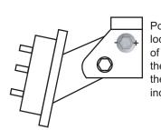
Point the - (Minus) located on the flange of the cam towards the outside of the vehicle to increase negative camber
